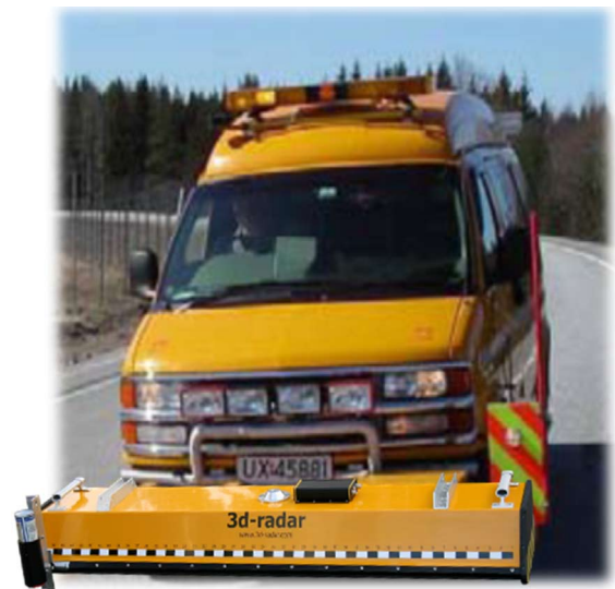
Figure 9: 3d-Radar GPR being used in road/bridge survey applications.
