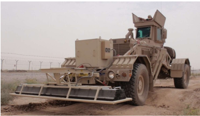
Figure 7: 3d-Radar GPR mounted on a Husky mine clearance vehicle.
